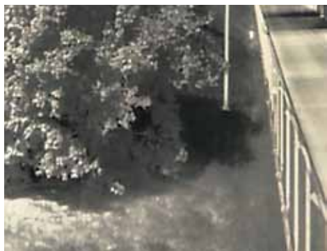
Branches moving in the wind caused many unwanted alarms in this location, so the head of security decided to replace the CCTV camera with a thermal imaging camera. Not one unwanted alarm has occurred since.
