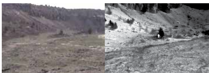
In most cases, thermal energy travels through the atmosphere more effectively than visible light. As a result, thermal imaging security cameras can spot intruders at extreme ranges while CCTV cameras, which rely on color contrast, will fail.
