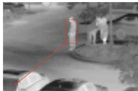
The FLIR Sensors Manager video analytics software has detected an intruder on the thermal image
